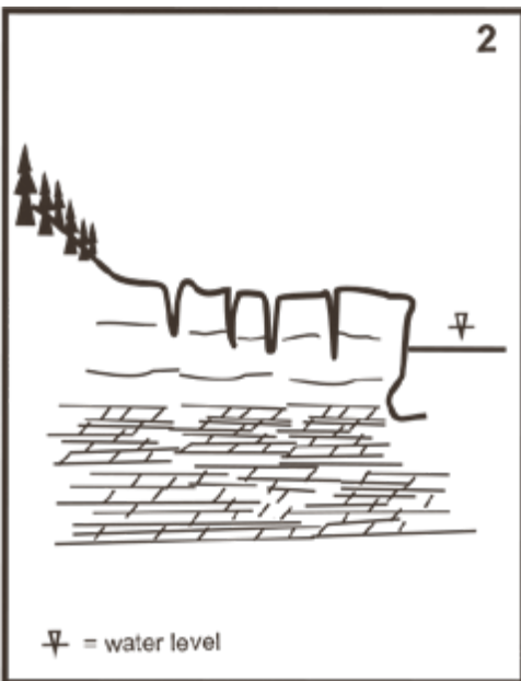
Diagram 2: As water levels recede further, waves begin to attack the edge of the shelf as well as lower layers. Joints are a critical component allowing the waves access to the rock mass enhancing the separation process.
